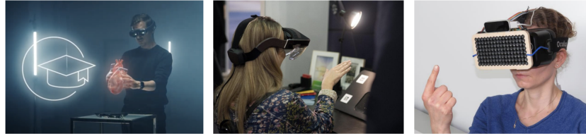
Fig. 3: Left: Tactile bio-hologram by [58]. Middle: AR car design simulation and customization demo by [59]. Right: VR with a head mounted mid-air haptic array by [57].
