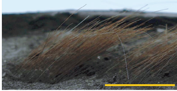
Fig. 7. Fake hairy skin made of silicon and graphite with fake hair grafted. Scale bar is 1 cm.
