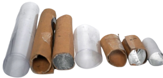
Fig. 9. Different electrodes tested (left to right): plastic, cardboard, cardboard with tinfoil, plastic, cardboard, cardboard with tinfoil and plastic with tinfoil.
