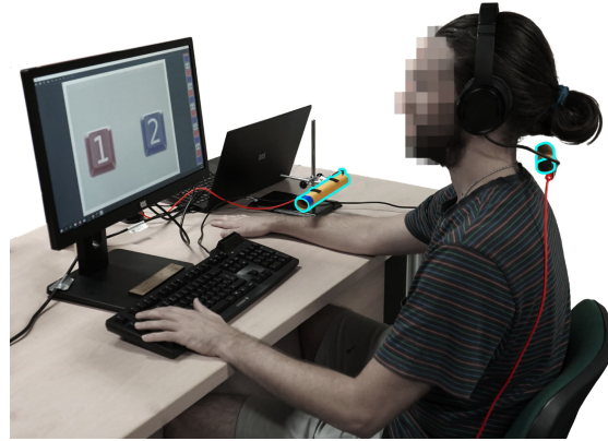
525 526 527 528 529 530 531 532 533 534 535 536 537 538 539 540 541 Fig. 13. Experimental setup for the user study of perception thresholds. There is an electrode above the forearm and above the nape 542 (separation 3.5 cm). The user is in front of a computer to report the perception of the stimulus. 543
